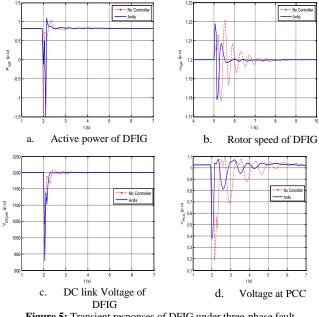
Figure 5:. Transient responses of DFIG under three-phase fault
